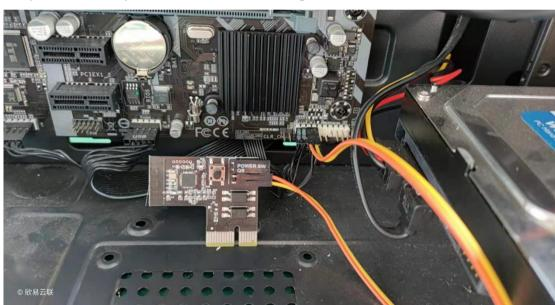
5.Locate the PCIE slot (generally behind the chassis with a baffle in the middle of the slot)
