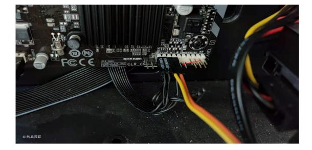
3.Connect the other end of the DuPont line to SW on the product; as shown in the figure below (no required)
