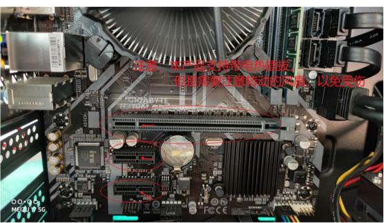
6. If the line on the computer POWER SW is too short, you can use the free extension line, the effect is as follows: Note: this product supports live hot-plug, but we need to pay attention to the rotating fan, so as to avoid cutting!!!
