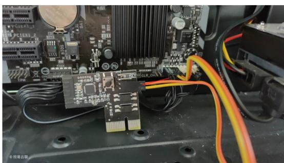
4. Connect the connector for the POWER SW removed from the motherboard to the product P-KEY position; as shown in the figure below  $\frac{1}{2}$
